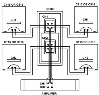
When the systems are connected in this way, it provides the best match of sensitivity and power handling between the CS265 and C115 or C516 satellites, whilst maintaining a nominal overall impedance above 4 ohms.
